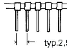
Ø hole in PCB typ. 1,0 mm
