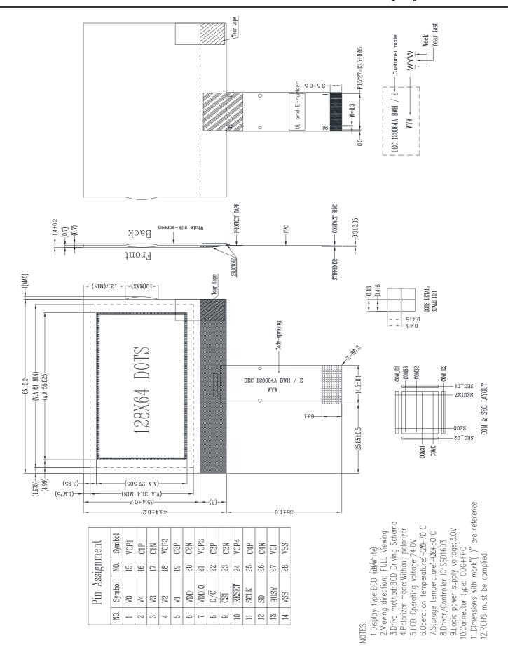
Figure 1: Module Specification
