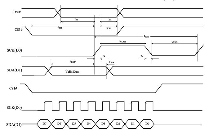
Figure 4: Timing characteristic of 4-wires Serial Interface
