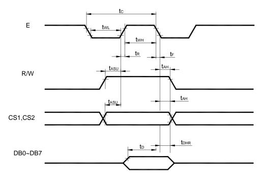
Figure 6.0 MPU Read timing
