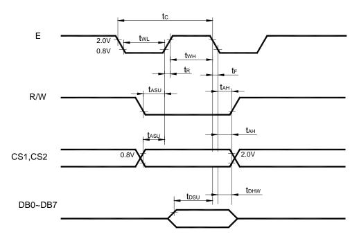
Figure 5.0 MPU write timing
