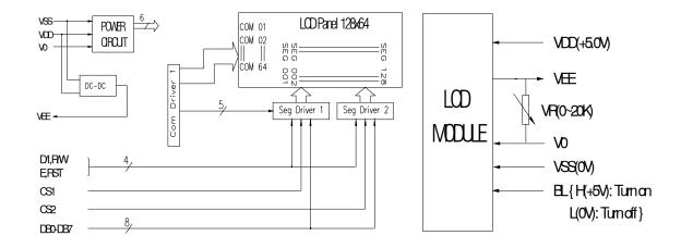
Figure 1. Block diagram
