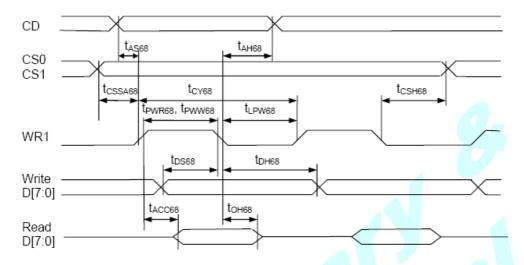
FIGURE 14: Parallel Bus Timing Characteristics (for 6800 MCU)  $(2.5V \le V_{DD} < 3.3V, Ta = -30 \text{ to } +85^{\circ}\text{C})$
