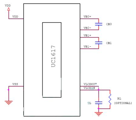
Reference circuit using internal Hi-V generator circuit
