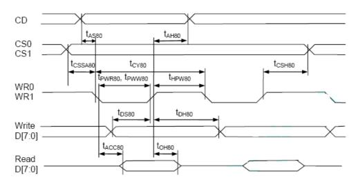
FIGURE 13: Parallel Bus Timing Characteristics (for 8080 MCU)
