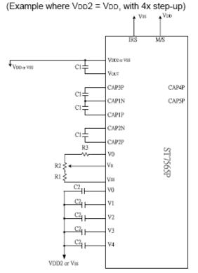
NOTE: Reference circuit used 4 times booster circuit.
