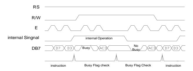
Example of 4-bit bus mode timing diagram
