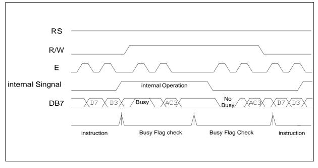
Example of 4-bit bus mode timing diagram
