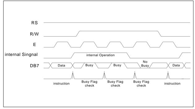
Example of 8-bit bus mode timing diagram
