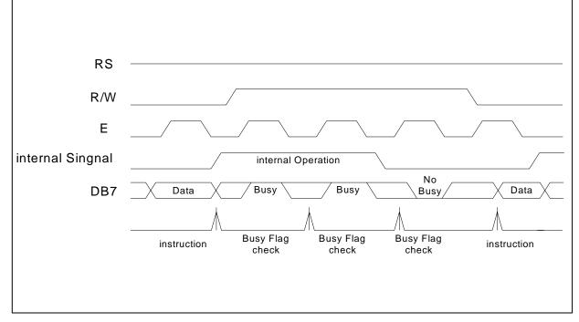
Example of 8-bit bus mode timing diagram
