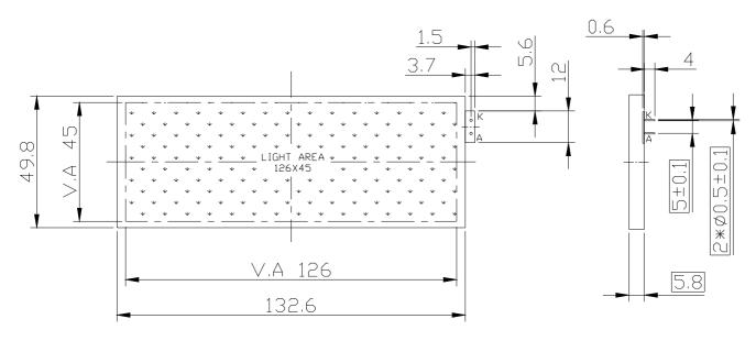
REMARKS: 1,UNMARKED TOLERANCE IS ±0.3, 2,ALL MATERIAL COMPLY WITH ROHS, 3,COLOR : YELLOW-GREEN. 4.Electronics/Optical Specifications:
