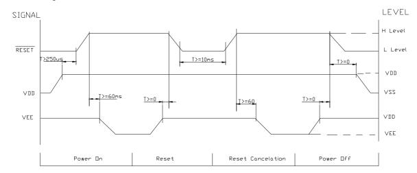
Please maintain the above sequence when turning on and off the power supply of the module.
