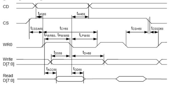
**Parallel Bus Timing Characteristics (for 6800 MCU)**
