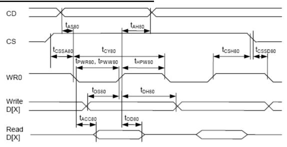
Parallel Bus Timing Characteristics (for 8080 MCU)
