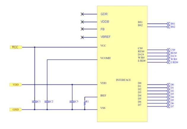
Recommended components: C1, C2 : 2.2uF/25V/0603 C3 : 1.0uF/16V/0603
