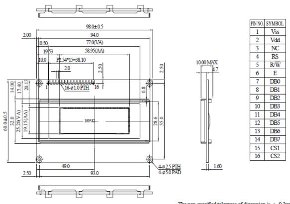
The non-specified tolerance of dimension is ± 0.2mm
