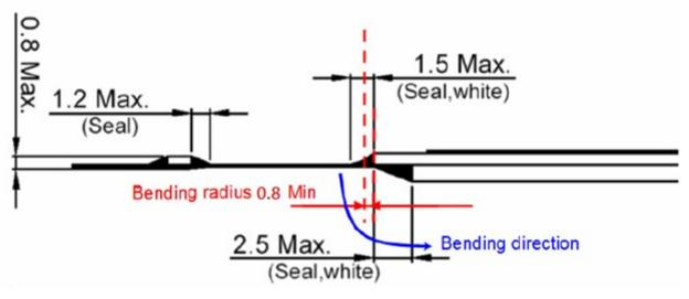
12.5 Avoid bending the film at IC bonding area.(>1.5mm)(this could damage the ILB bonding)
