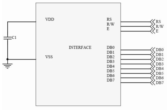
Pin connected to MCU interface: RS, R/W, E, DB0~7
