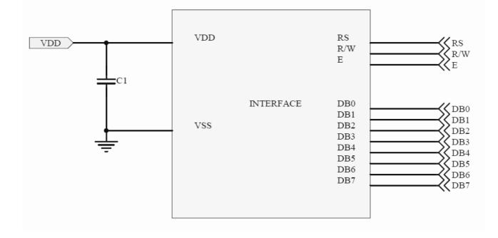
Pin connected to MCU interface: RS, R/W, E, DB0~7
